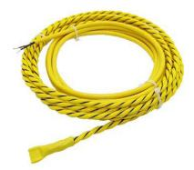
WLMC 2-Core leak detection ropes include a 2M lead wire, however this wire may be extended using alarm cable. The total length of lead wire and sensing cable may not exceed 30M. If more than 30M is required, use multiple WLM controllers.
