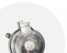
An air pressure differential switch is a mechanical switch fitted in ductwork which can be used to monitor and check airflow rates. These switches are adjustable and have a range from 20-300PA, they also come with a 1m duct kit to be fitted into the ductwork and detect the airflow.
