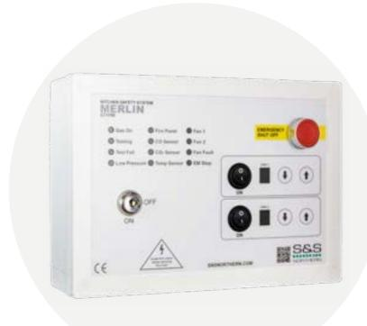
The Merlin CT1750 System is a gas interlock and manual ventilation control system designed for commercial kitchens. The Merlin CT1750 System comes with two variable fan speed controllers (0-10V output) to control the speed of 2 fans via an inverter.
